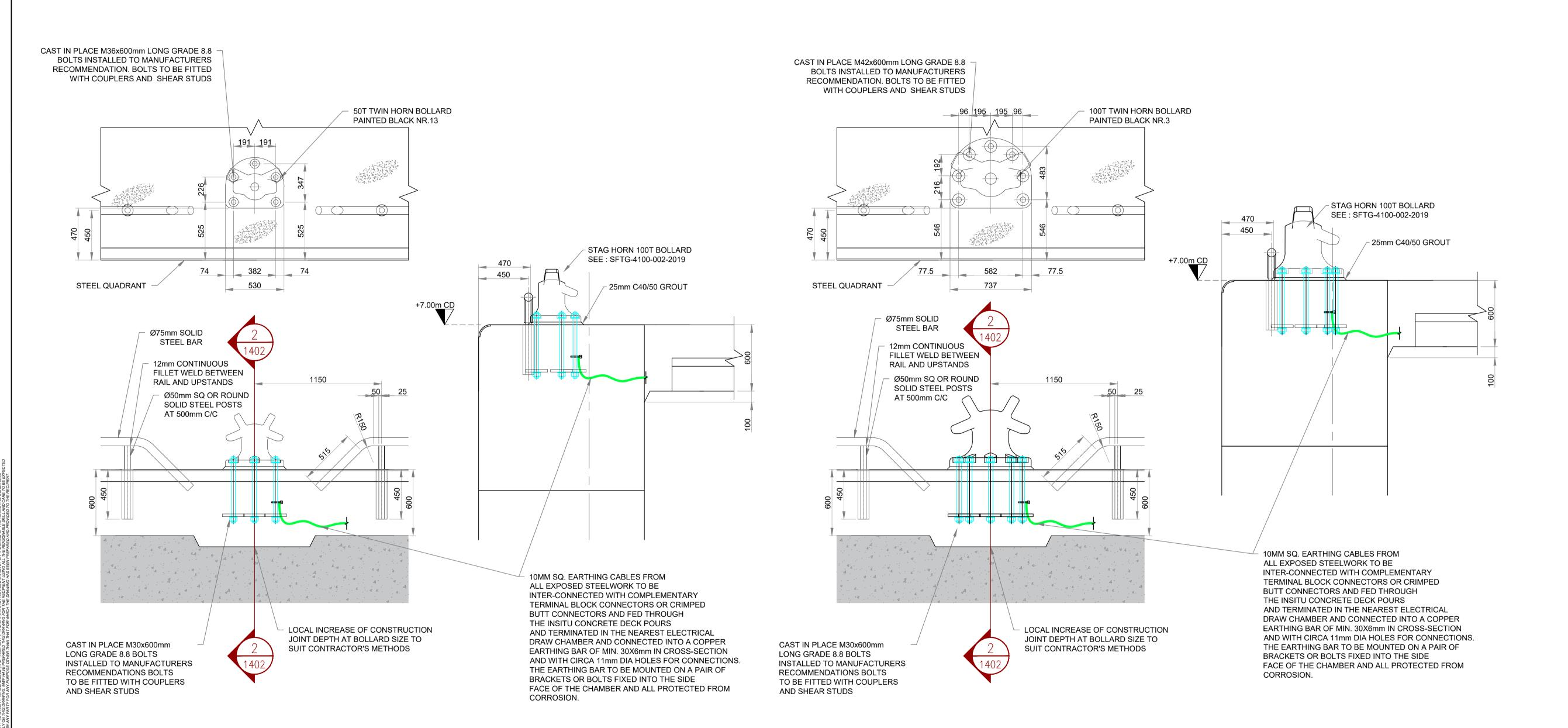
DETAIL 50t BOLLARD 13nr. SCALE: 1:20
